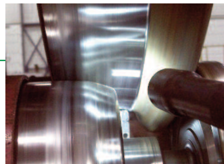
REPROFILING OF WHEEL (SOURCE: LLOYD'S REGISTER RAIL)
